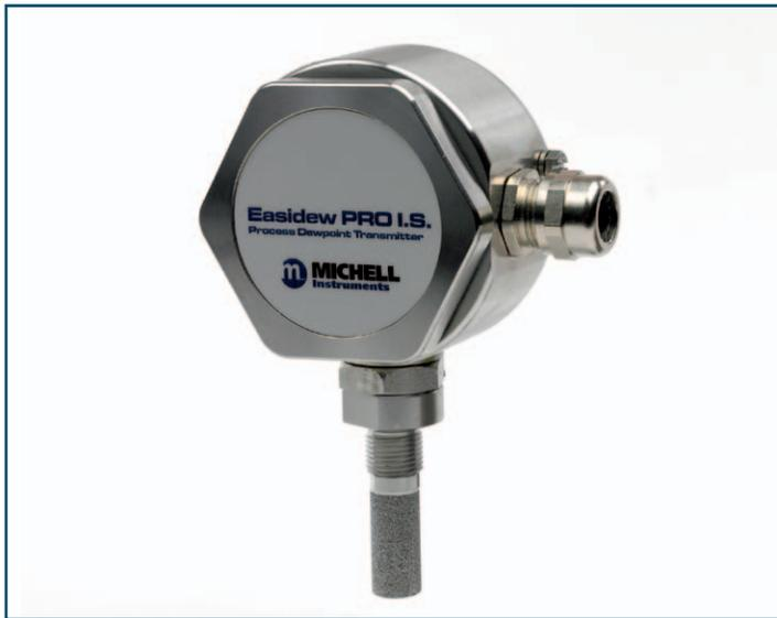
The Easidew PRO I.S. is a rugged intrinsically safe 2-wire dew-point transmitter for trace moisture measurement in liquids and gases. It is certified for use in Class 1 Div 1 Groups A,B,C and D, EXII 1G EX ia IIC T4 and I.S. I 1 ABCD T4 ( $T_a = +60^\circ\text{C}$ ) hazardous area locations.
